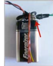
9V Batteries may need a rubber band around them to be secure
